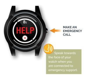
**IMPORTANT:** To cancel an accidental activation, press the **X** on the display prior to the countdown reaching zero.
